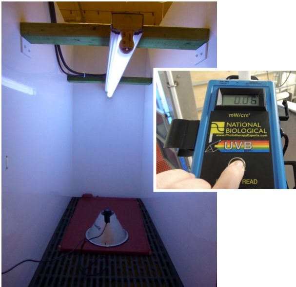
Station for exposing piglets to UVB light (left) . UVB meter (right) . Photos: AAFC Sherbrooke Research & Development Centre
