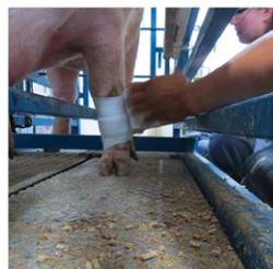
Wrapping an accelerometer onto the rear leg of a sow on a force plate scale.
