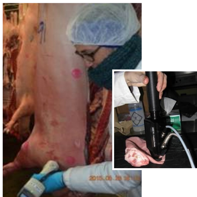
New technologies have shown promise in assessing meat quality. Left: Using a spectrophotometer on a pig ear to assess bruising colour. Right: Using NIRS on pig ears. Photos: AAFC
